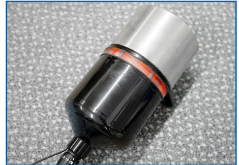
Deploy the sensor and ensure the vanwaltKISS device is secure at the top of the well. Do not drop/force the sensor.
