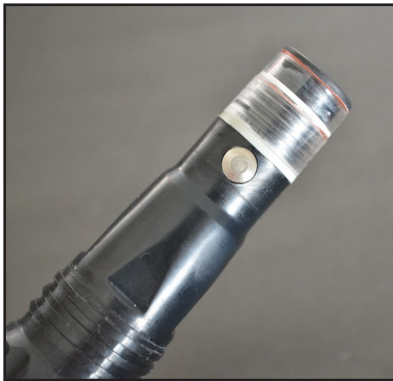
Figure 2: Thermistor & sensor cap
