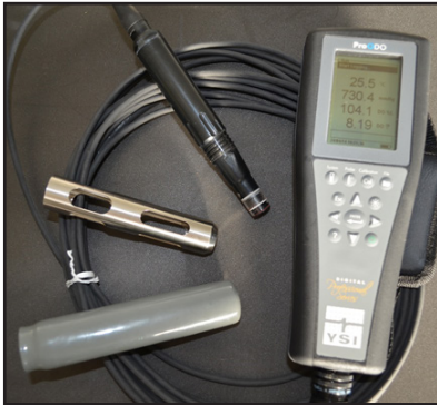
Figure 1: Clockwise from bottom left - Grey transport sleeve, silver sensor guard, sensor, ODO handset
