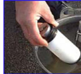
Taking care not to damage piston rings, carefully push & twist sample tube & insert into frame. Place collar at top of frame. Check that piston rod & hole are in line, if not rotate collar by 180°. Tighten wing nuts firmly & check tightness of these after taking each sample.
