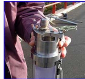
Push piston rod through collar & screw into piston loosely.
