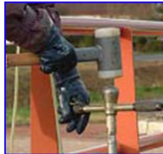
Once required depth is reached replace air hose in pressure pump & apply 2, to no more than 3 bars pressure. Gradually pull sampler upwards in a straight line.
