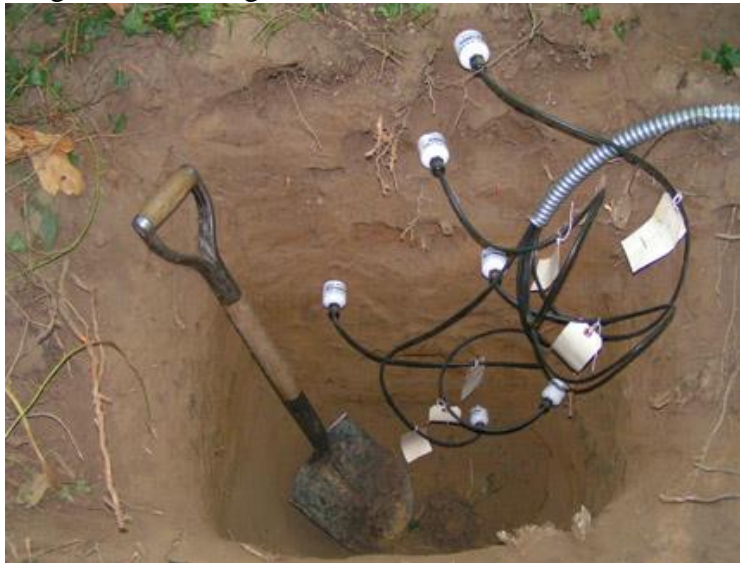
Figure 2.3 Six HydraProbes installed into 6 distinct soil horizons.
