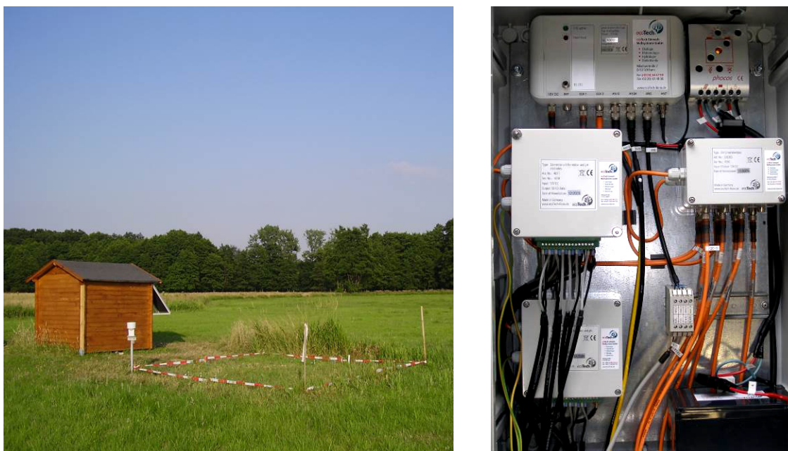
Fig. 10: Field station for the investigation of As concentration in the soil water as affected by redox potential, pressure head and soil temperature; measurement and automatic data acquisition with 18 redox electrodes, tensiometers, temperature sensors and soil water extraction by suction cups in 6 soil depths
