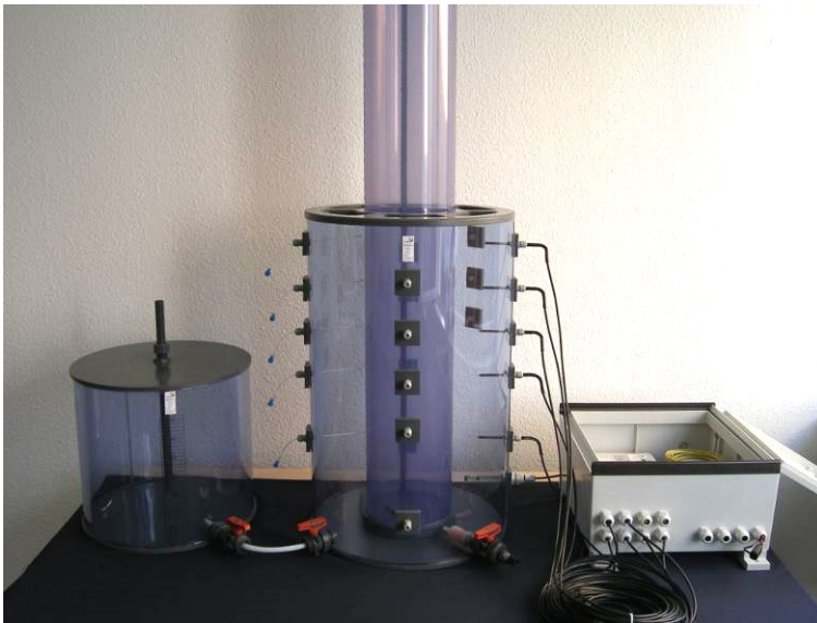
Fig. 11: Laboratory setup for the measurement of redox processes in the soil water as affected by the redox potential, pressure head, and soil temperature
