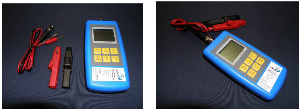
Fig. 12: Equipment for mobile measurements of the redox potential: Handheld for redox, pH and temperature (Art. No. 4612) as well as an adapter with connectors for the cable ends of the electrodes (Art. No. 4613)
