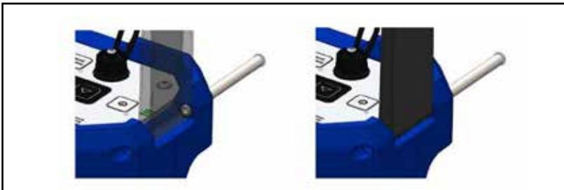
4. Push the carrying strap pin back into position using the hex key, while twisting clockwise if necessary.
