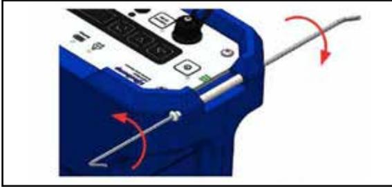
2. Remove the carrying strap pin by pressing it out of the housing chamber with the hex key. Push the pin out of the hole until it reaches the position shown.
