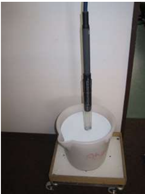
Fig.: PICO T3 probe head inserted in a TECANAT calibration tube which again is installed in dry glass beads. Make sure that the tube probe's wave guides are completely inserted into the glass beads when measuring. The basic alignment will fail if the wave guides are in part surrounded by air.
