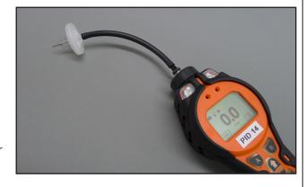
The PID is a gas detection device. It is not designed to suck in moisture or sediment. The "moisture filter" enclosed in the filter clamp assembly on the top of the unit is designed to stop moisture and sediment moving into the machine and should be replaced regularly and also when it appears necessary. This is a prudent move to maintain the PID without problems.
