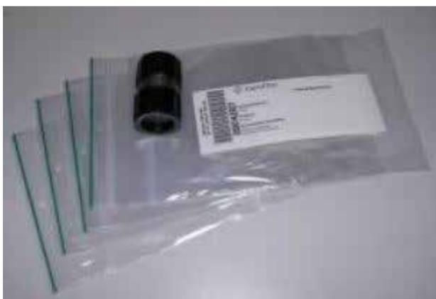
Take a duplicate\*\* sample to allow the lab to express the concentrations measured as based on dry weight
