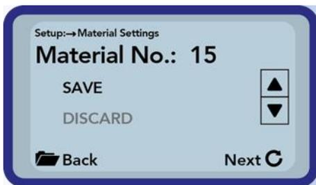
Finally, you can store the calibration into the chosen calibration storage inside the probe. Choose „SAVE“ and confirm by pressing the button „Measurement“
