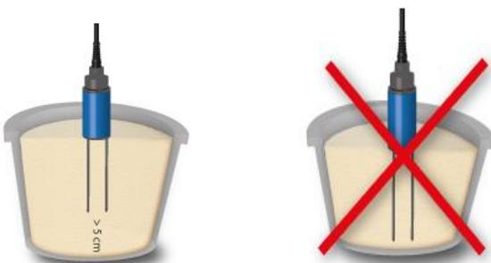
The HD2 Kit is high precision measurement device. Carefully follow the above requirements to achieve repeatable, reliable and precise results from your measurements.
