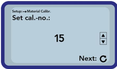
First you have to set the calibration curve to be changed (01 – 15) by pressing the buttons „Up“ ▲ and „Down“ ▼. Apply your setting by actuating the button „Measurement“ C.
