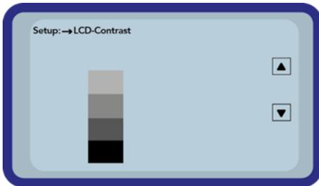
Change the contrast by actuating the button „Up“ ▲, respectively „Down“ ▼. Set the contrast that you can realize the whole grayscale on the diagram. Activate and store your settings by actuating the button „Measurement“ Ⓞ. After activation, the symbol 📄 will appear in the upper right hand corner of the display.
