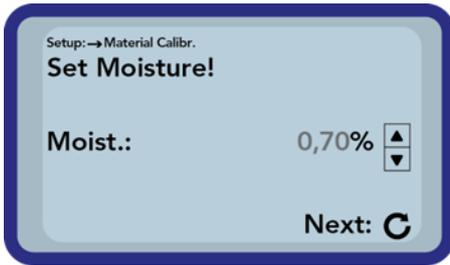
Next set the moisture of the material by pressing the buttons „Up“ ▲ and „Down“ ▼. Apply your setting by actuating the button „Measurement“ C.
