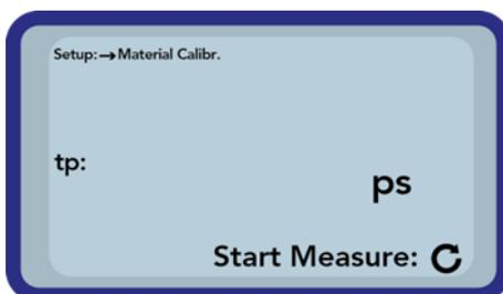
To start the measurement of the material press the button „Measurement“
