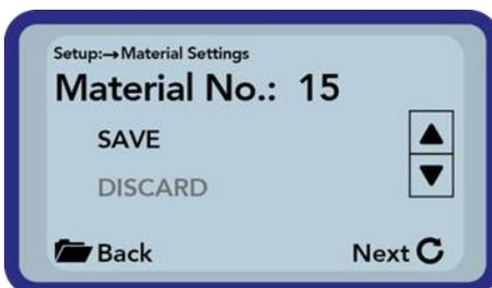
Finally, you can store the calibration into the chosen calibration storage inside the probe. Choose „SAVE“ and confirm by pressing the button „Measurement“ C. If you choose “DISCARD” everything is left untouched.
