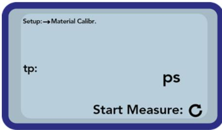
To start the measurement of the material press the button „Measurement“
