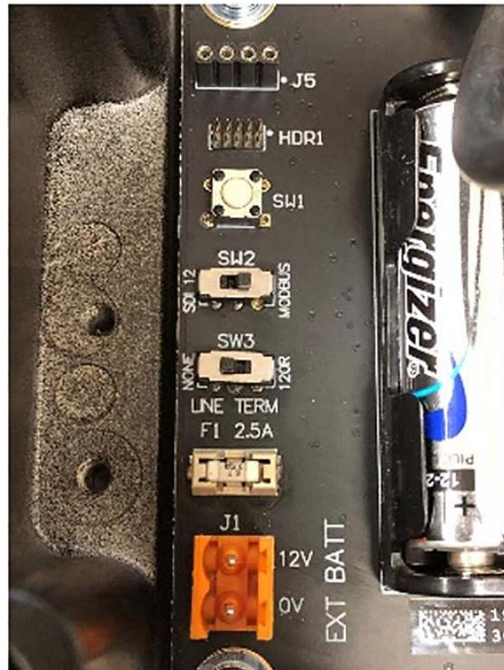
Figure 3 Fuse, switches and button
