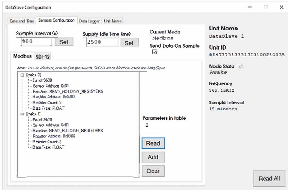
Figure 17 Sensor Configuration
