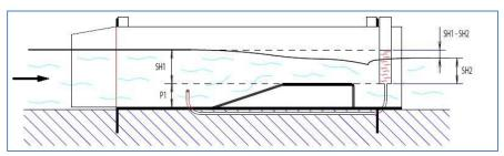
designed for use in smaller water ways or earthen channels (irrigation channels, in- outlets, furrow, ditches, etc.). The RBC flume is a simple and reliable instrument for the measurement of the quantity of irrigation water that flows towards a field. Using standard formulae the flow through quantity (the discharge) is calculated. Instead of reading the stilling well it is possible to install a pressure transducer connected to a datalogger
