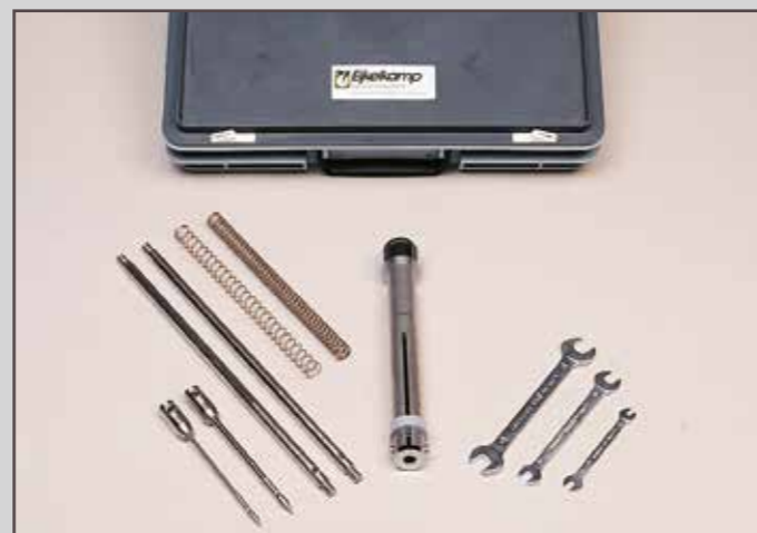
Penetrometer for Top Layers
