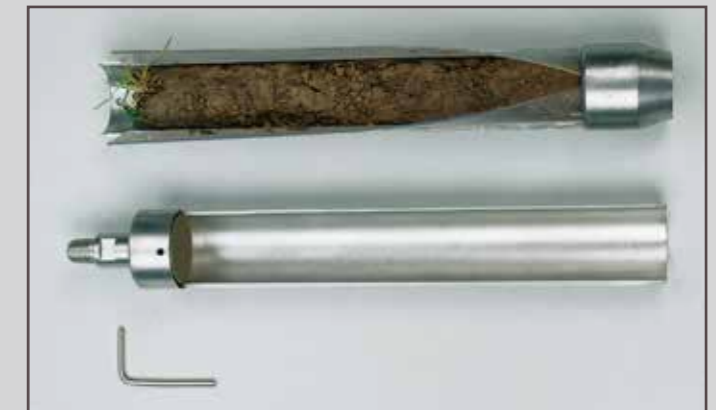
Split tube sampler for top layers
