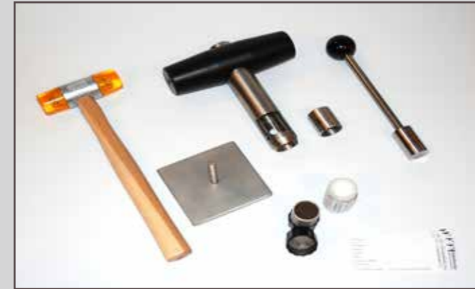
No-Loss Soil Corer
