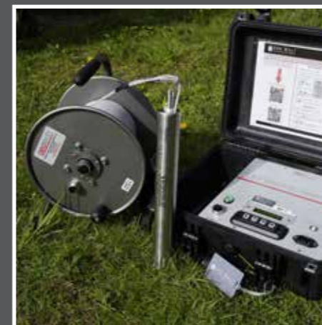
Geosub Pump & Controller
