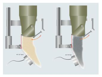
The red arrow indicates how the opening flap of the silo should be located under the upper edge of the baffle plate so that the probe is not just partially but completely covered by material.
