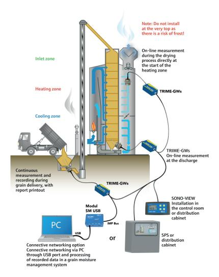
TRIME-GWs can be used in various fields of application. They can, for example, be used to monitor the moisture of the delivered grain or to support or automate grain drying. Depending on the type and density of the grain to be measured, the appropriate calibration curve must be selected.
