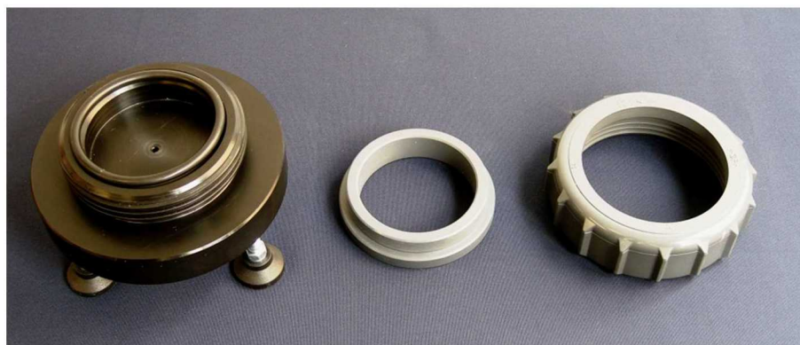
Figure 2: Build-up of column base for tubes with ID = 65 mm und ID = 50 mm. From left to right: Column base with O-ring, clamp ring/collar, fastener-clamp ring system for the large leaching column and ring/union nut.
