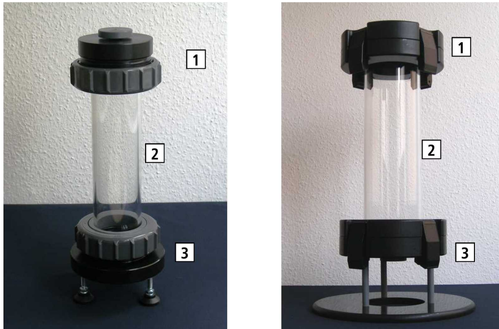
Figure 1: Leaching columns (on the left ID 65 mm; on the right ID 100 mm) with column lid (1), glass tube (2) and column base (3)
