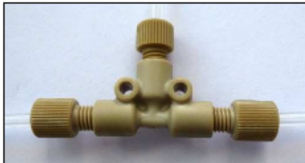
Figure 3: Tee connector between pump, pressure sensor and leaching column
