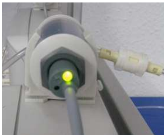
Figure 6: Saturation sensor with control LED
