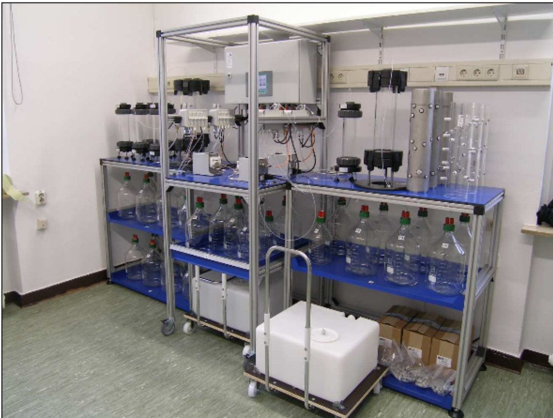
Figure 1: Installation with four columns housed in its three part rack system (center rack and two end racks) with its individual modules (1: eluent reservoir; 2: pump; 3: leaching columns; 4: hydraulic distributor; 5: sampling bottles)
