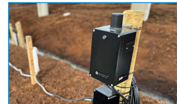
Self-powered, wireless Datalogger - capable of networking up to 30 inputs, across multiple parameters
