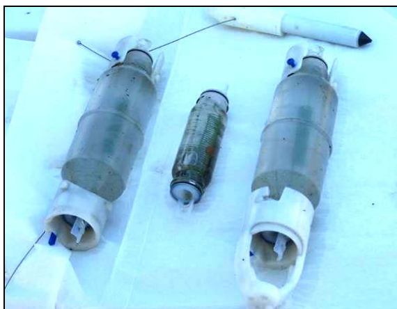
Figure 5-6. Snap Sampler samples showing black particles and piece of rusted casing (inside VOA vial).
