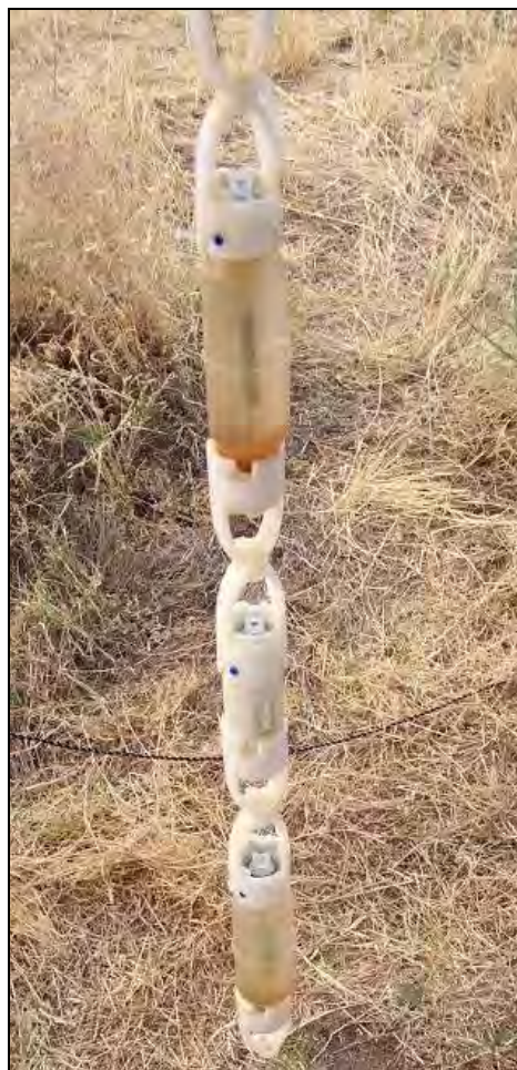
Figure 5-7. Snap Samplers containing an orange precipitate.
