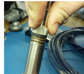
Push top cap in before twisting and locking
