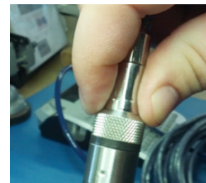
Properly completed—black ring uncompressed
