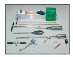
A **Root Auger Set** for obtaining virtually undisturbed, uniform soil samples for root system analysis to a depth of 2 meters.
