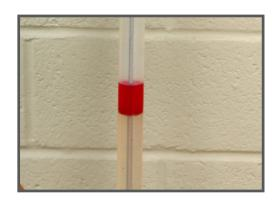
**Liquid Layer Sampler** an easy to use sampler to capture a product/water interface.
