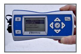
**e+CONTROL** is an easy to use, field use reader and programmer for Diver and all e+ Sensors.
