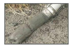
**Beeker Sampler** used to take undisturbed samples of sediments and submerged soils.
