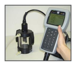
The **YSI 556** is a Multi Parameter Meter capable of measuring up to 10 different parameters simultaneously.
