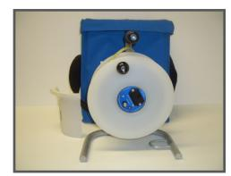
The **Water Level Meter** uses a 16mm probe to measure depths in wells to an accuracy of 3mm.
