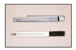
**Vrijwit Auger** a perfect auger for taking samples from shallow water bottoms with roots.
