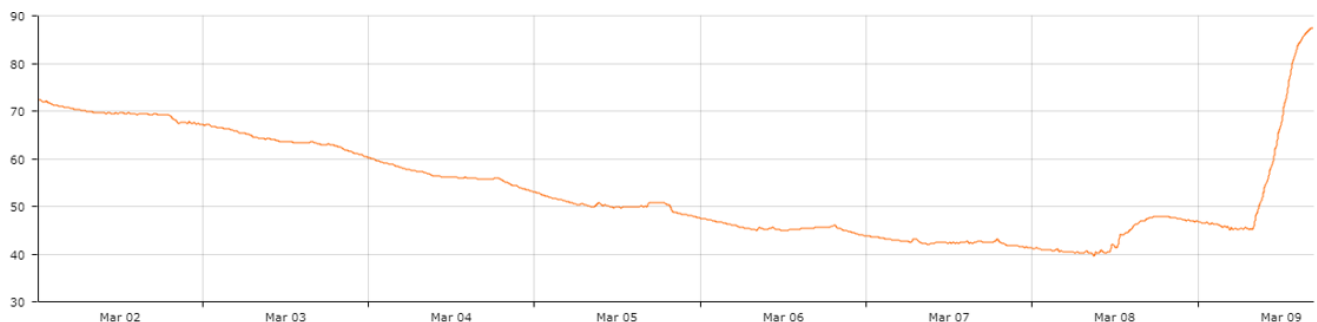
Figure 3 - Example flow output from flume with Van Walt Data Collection system
