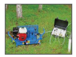
**Total Fluids Pump - Reclaimer** an externally controlled compressed air operated pump for well development, purging and remediating.
