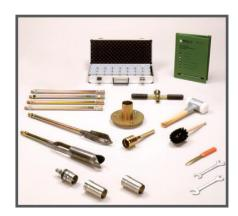
Soil Sample Ring Kits for the collection of undisturbed soil samples in rings of uniform dimensions for analysis in the laboratory.
