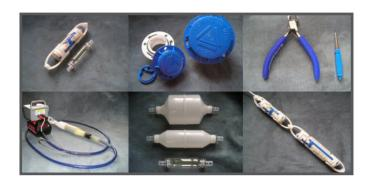
**Snap Sampler** a passive groundwater sampling approach that seals groundwater samples onsite.
