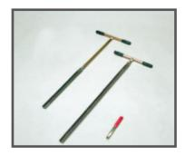
**Single and Extendable Gouges** for soil mapping, suitability reviews, root, fertilisation, clay and paleontological research with minimal disturbance.
