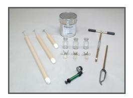
**Samplers with ceramic cup** are soil moisture samplers with ceramic cup ideal for sampling low interaction chemicals like nitrates.
