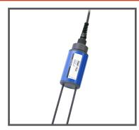
**Pico 64** a highly sophisticated TDR probe for onsite monitoring of soil moisture in top layers.
