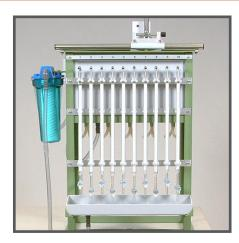
A **Permeameter** is used to establish the permeability of soil for irrigation and drainage sytems, well pumping, subsidence investigations, predicting the spread of polluting fluids, soil improvement and maintenance advice.
