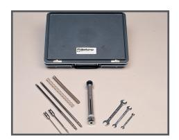
A hand held **penetrometer** for the determination of the penetration resistance of top layers
