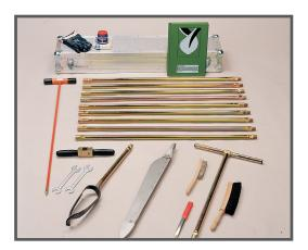
**Peat or Russian Corer** easy to operate, manual corer for sampling at different depths in sediment and wet soils, including below the groundwater level.
