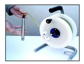
The **GT Oil Interface Meter** uses a 16mm probe to detect hydrocarbons as thin as 1.52 mm in wells as small as 19mm in diameter.
