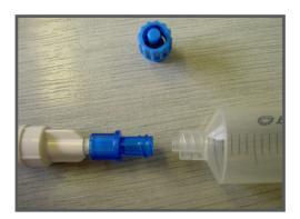
**Macro Rhizon** for soil moisture sampling in the field when successive soil solution samples are needed from the same volume of soil.
