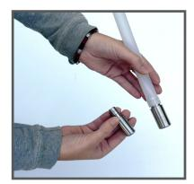
**Footvalve Pumps** an economical, manual pump for environmental analysis available in diameters from 9mm to 22mm.
