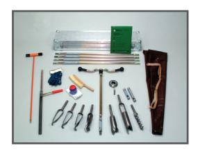
The **Ergonomic Auger Set** is used to carry out manual drilling and sampling in a great variety of different soils in an ergonomically sound way. It can help prevent back, neck and shoulder problems which can be associated with repetitive augering.
