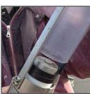
Push piston rod through collar & screw into piston loosely.
