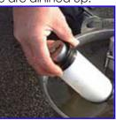
Taking care not to damage piston rings, carefully push & twist sample tube & insert into frame. Place collar at top of frame. Check that piston rod & hole are in line, if not rotate collar by 180°. Tighten wing nuts firmly & check tightness of these after taking each sample.
