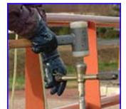
Once required depth is reached replace air hose in pressure pump & apply 2, to no more than 3 bars pressure. Gradually pull sampler upwards in a straight line.
