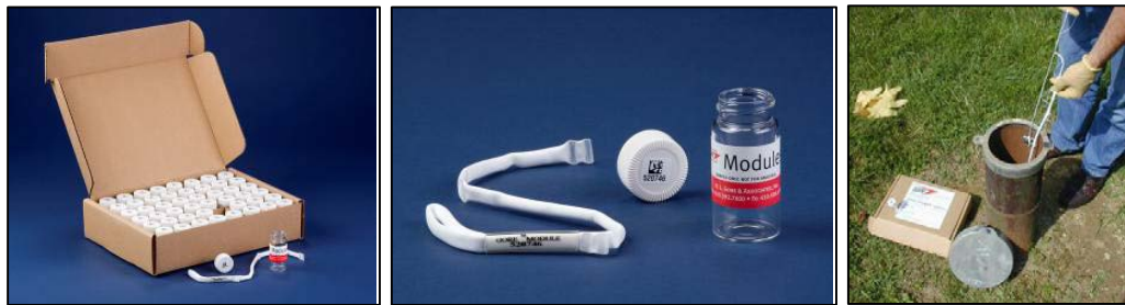
AGI Universal Sampler – A Sorptive Sampler
