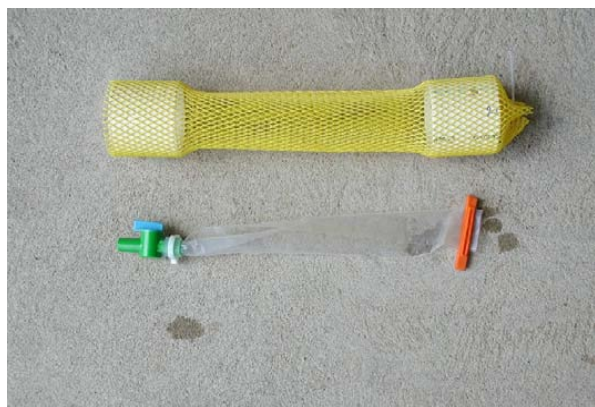
Regenerated Cellulose Dialysis Membrane Equilibrium Sampler
