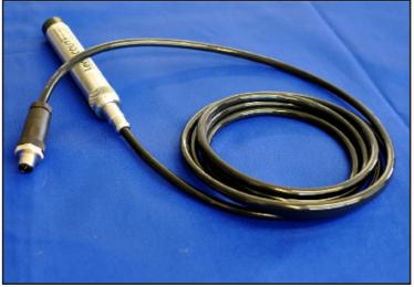
Direct read cables need to be robust, reliable, non stretch and this is why the LevelSCOUT 2X cables are so ideal for the purpose. The connectors, either in stainless steel or titanium are very robust and, because they have a swaged fitting, they are rated for very deep submergence. The cables themselves, available in several materials (including Teflon) and with or without Kevlar reinforcement are bigger and more robust than most competing cables.
