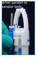
Push release pin up through hole in Snap Cap
