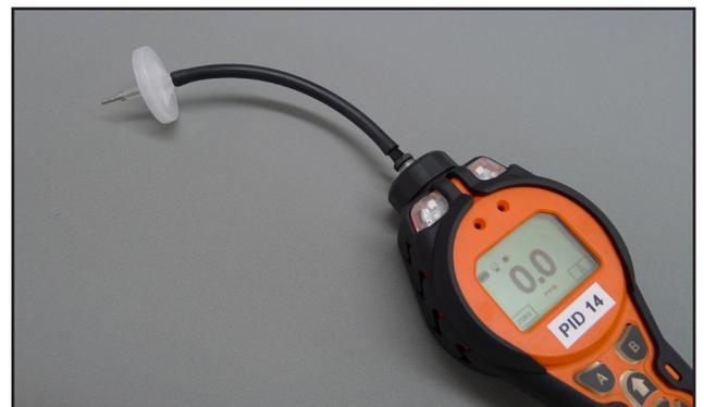
The PID is a gas detection device. It is not designed to suck in moisture or sediment. The "moisture filter" enclosed in the filter clamp assembly on the top of the unit is designed to stop moisture and sediment moving into the machine and should be replaced regularly and also when it appears necessary. This is a prudent move to maintain the PID without problems.
