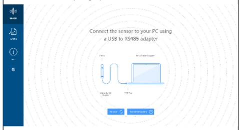
If your cable and sensor were not connected before opening Aqua4Plus 2.0 simply connect and click Rescan. While scanning is active you'll see a green dot flash in the upper right corner of the program. Scanning is complete when this dot stops flashing.
