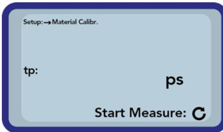
To start the measurement of the material press the button „Measurement“ C. To improve the accuracy, four measurements will be taken.
