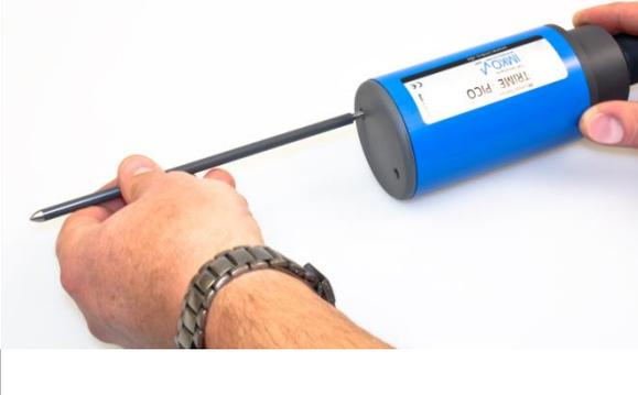
A hand holding a metal rod and screwing it into the front of the blue probe body. |
