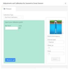
Aqua4Plus 2.0 will take 10 readings and display the average. Watch for stability while the software is measuring to ensure an accurate calibration.
