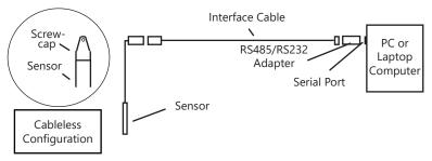
Connect the sensor to your computer using an RS485/RS232 adapter and an interface cable.
