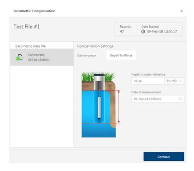
Aqua4Plus 2.0 will perform the barometric compensation and create a new compensated report. Original reports are retained as uploaded.
