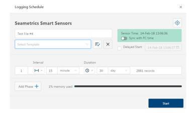
Click to switch between interval and continuous data recording (PT2X & CT2X only) Select your continuous rate from the drop down box (on the right).
