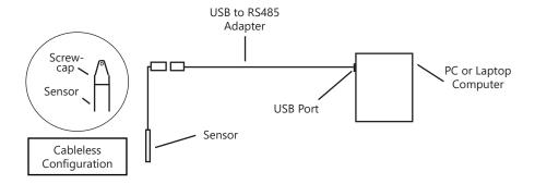
Connect the sensor to your PC using Seametrics' USB to RS485 adapter.
