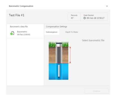
If compensating for Depth to Water enter your depth to water reference measurement and the date/time the measurement was taken (typically taken with a water level indicator before data is uploaded from the sensor) before clicking Continue.
