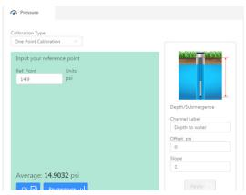
Click Apply to confirm settings and Aqua4Plus 2.0 will provide a real time reading to confirm.
