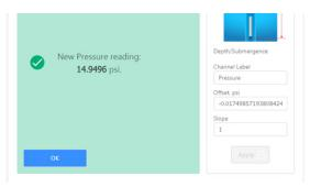
2 Point submergence calibration **ONLY RECOMMENDED IF YOU HAVE AN ACCURATE PRESSURE REFERENCE**. Our Smart Sensors rarely change slope during normal use, however if you have an accurate pressure source it is possible to perform a 2 point calibration on the pressure channel.
