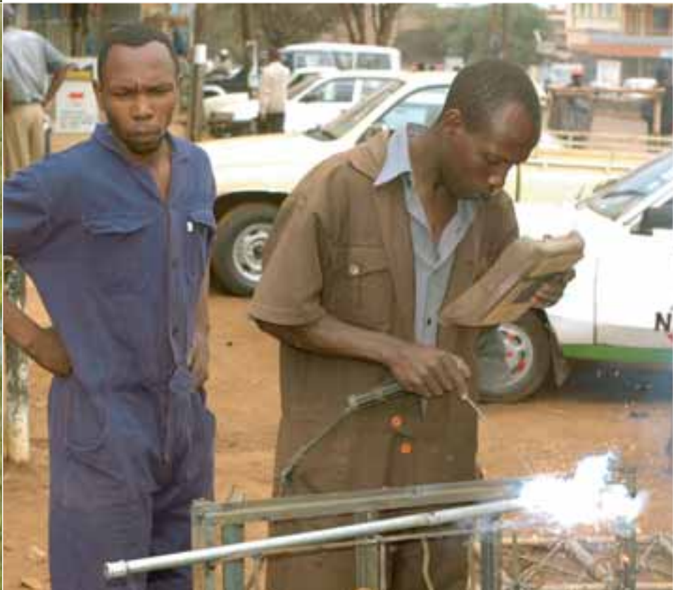
Manufacturing a primitive peat auger on the streets of Nyeri (Kenia)
